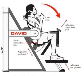
\* Feet and pelvic position is adjusted in raport with subject height, to get an angle of approximately 90 degrees between thighs and calves.
